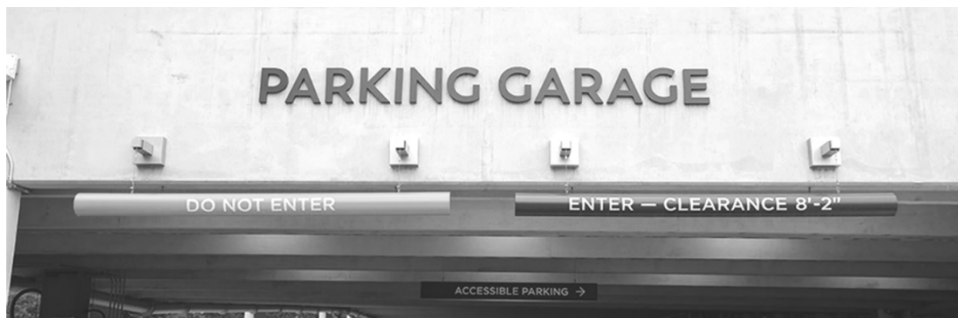
Figure. 2.2 Height clearance bar and height limits
